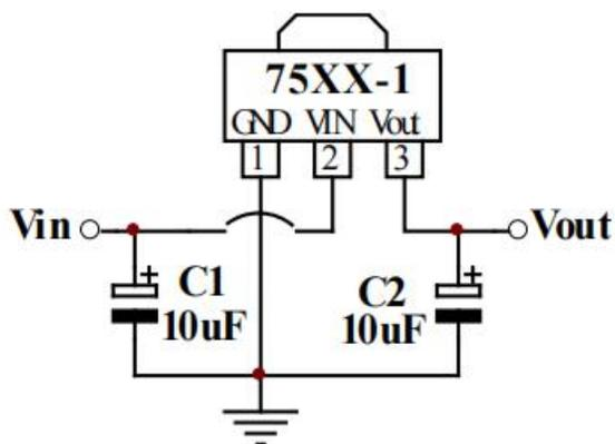
High Output Current Regulator Circuit 高输出电流稳压电路
